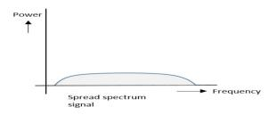
5. This is frequency hopping technique, where the users are made to change the frequencies of usage, from one to another in a specified time interval, hence called as **frequency hopping**. For example, a frequency was allotted to sender 1 for a particular period of time. Now, after a while, sender 1 hops to the other frequency and sender 2 uses the first frequency, which was previously used by sender 1. This is called as **frequency reuse**.
